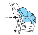
be no more than one inch (2.5 cm) of movement for proper installation.
